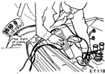
Fig. ET-8 Checking ignition timing
