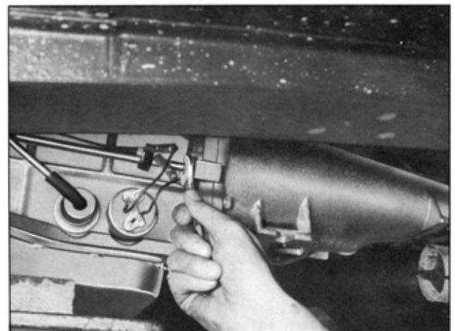
*Fig. TM-12 Removing oil cooler tube*
