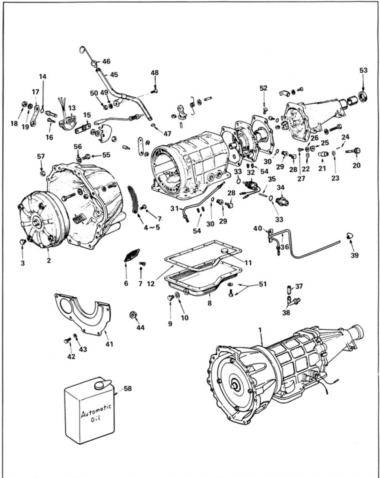
Fig. TM-2 Transmission case
