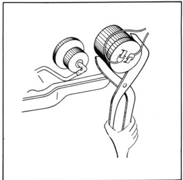
Fig. TM-6 Removing downshift solenoid
