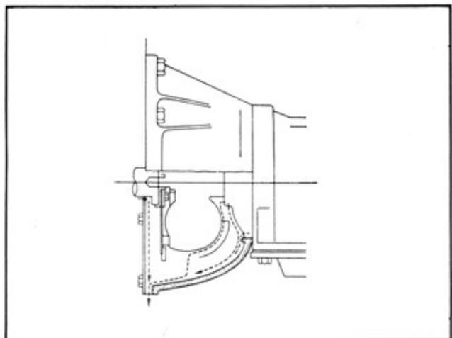
Fig. TM-4 Oil leak point of converter housing
