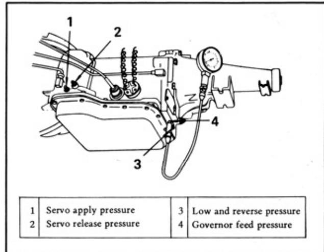
Fig. TM-9 Measuring line pressure
