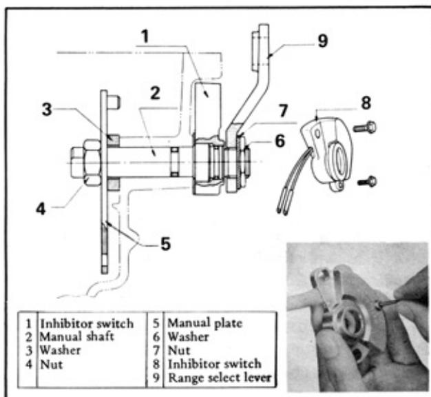
Fig. TM-8 Construction of inhibitor switch
