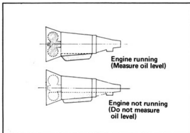
Fig. TM-3 Measuring oil level
