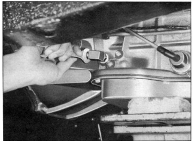
*Fig. TM-11 Removing oil cooler tube*
