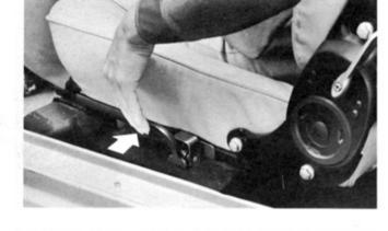
The seat back can be tilted to and fro while pulling the lever forward. To lock the seat back, release the lever and lock the seat back at a desired position.
