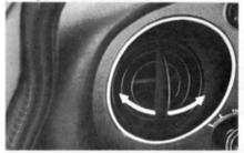
Co-driver's Side Ventilation Louver - Pull out the knob to open the air outlet, and move the lever to adjust air flow direction.
