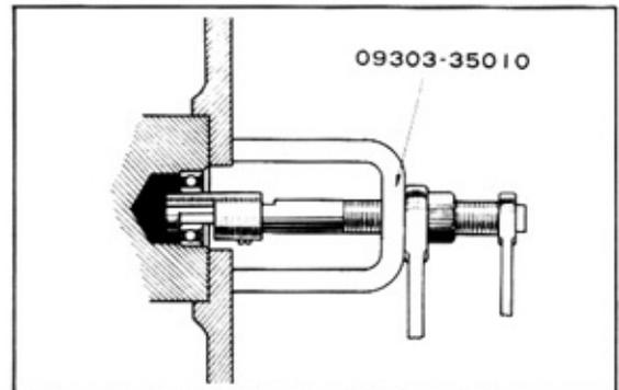
Fig. 1-26 Removing Bearing
