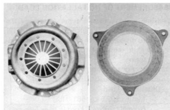
Fig. 1-23 Clutch Cover Inspection
