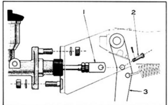
Fig. 1-12 Removing Master Cylinder
