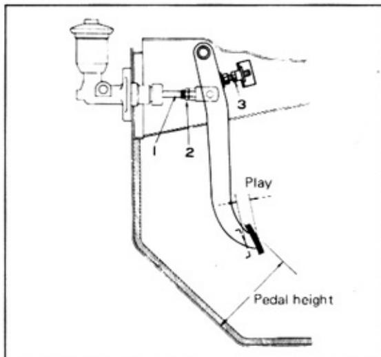
Fig. 1-2 Pedal Adjustment
