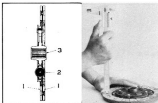
Fig. 1-21 Clutch Disc Inspection
