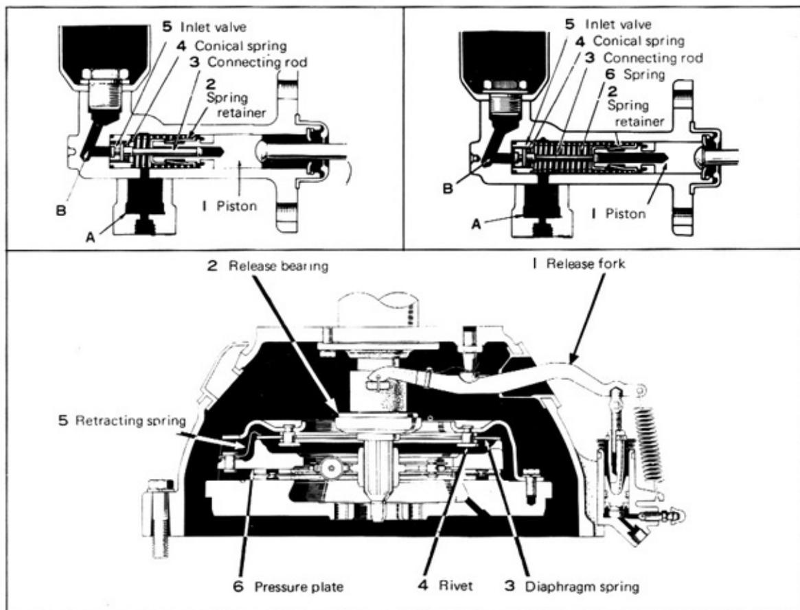
Fig. 1-1 Clutch System
