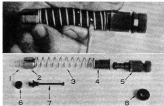
Fig. 1-14 Disassembling Piston
