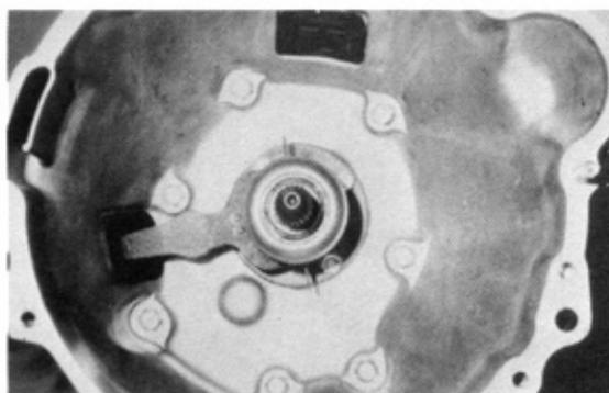
Fig. 1-29 Release Fork Assembly
