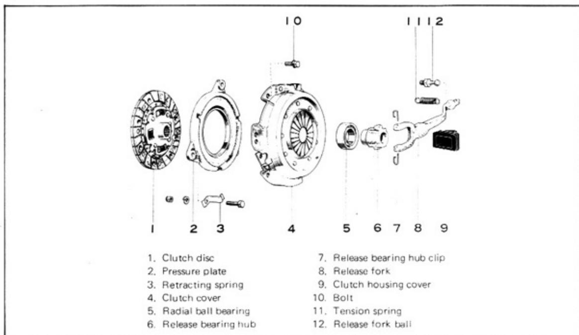
Fig. 1-17 Clutch Assembly
