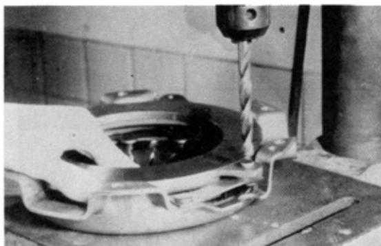
Fig. 1-20 Clutch Cover Disassembly
