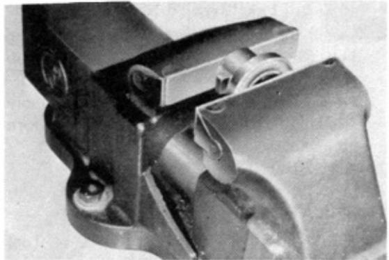
Fig. 1-25 Installing Bearing
