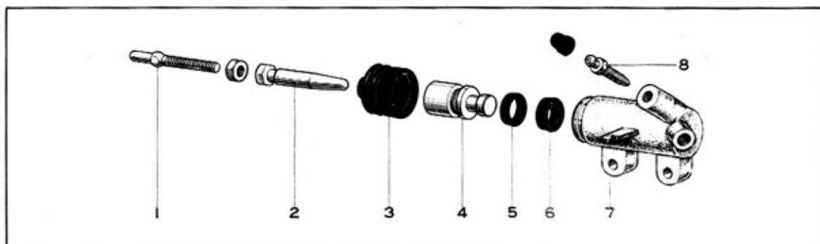
Fig. 1-8 Clutch Release Cylinder
