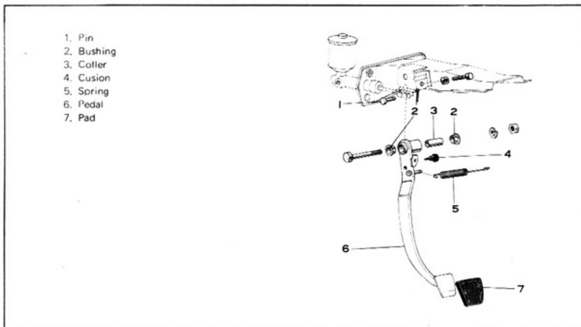
Fig. 1-5 Clutch pedal
