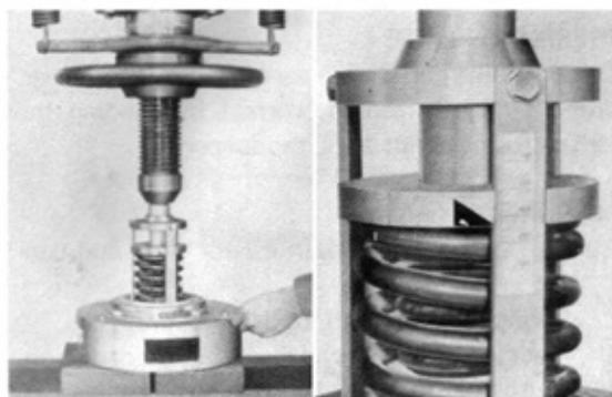
Fig. 1-19 Measurement of Installation Load
