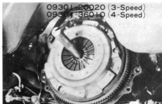
Fig. 1-30 Clutch Assembly
