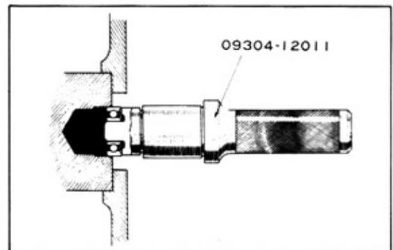
Fig. 1-27 Installing Bearing
