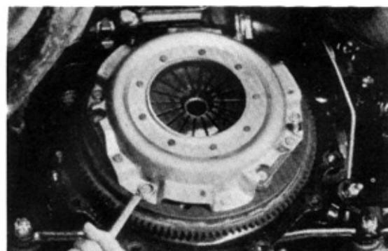
Fig. 1-31 Clutch Assembly
