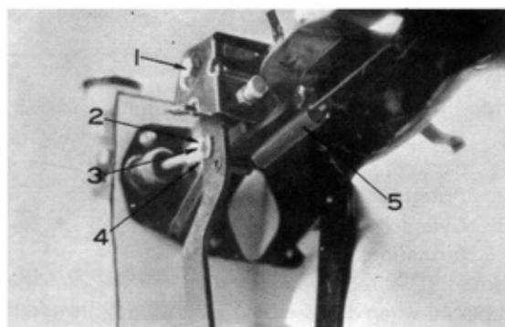
Fig. 1-6 Removing Clutch Pedal
