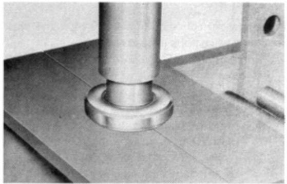
Fig. 1-24 Removing Bearing
