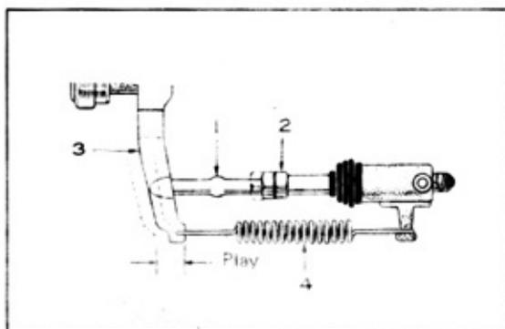
Fig. 1-9 Removing Release Cylinder
