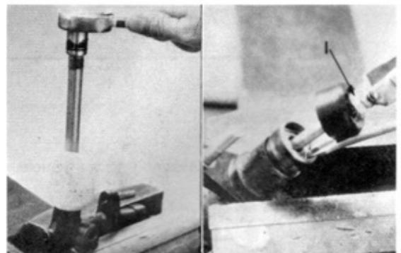
Fig. 1-13 Disassembling Master Cylinder
