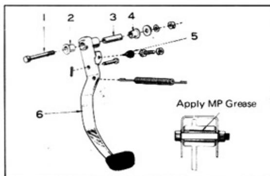
Fig. 1-7 Installing Clutch Pedal
