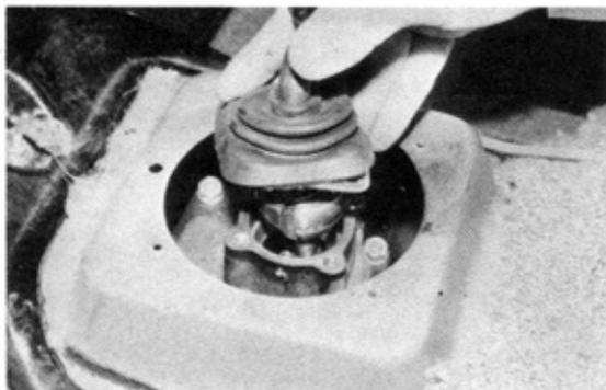
Fig. 2-145 Removing Shift Lever
