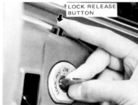
LOCK —The steering wheel is locked. The key can be removed only at this position.
