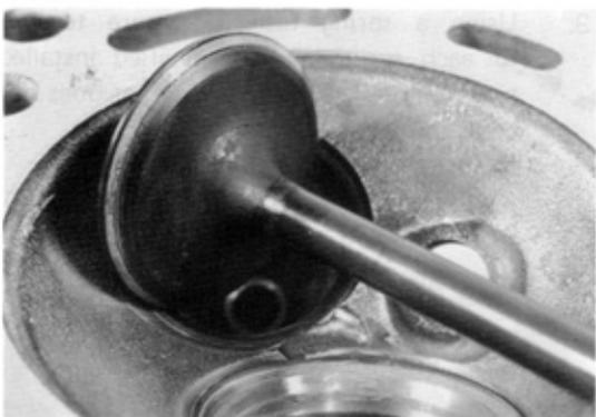
7. Resurface valve seats with 45° carbide cutter.
