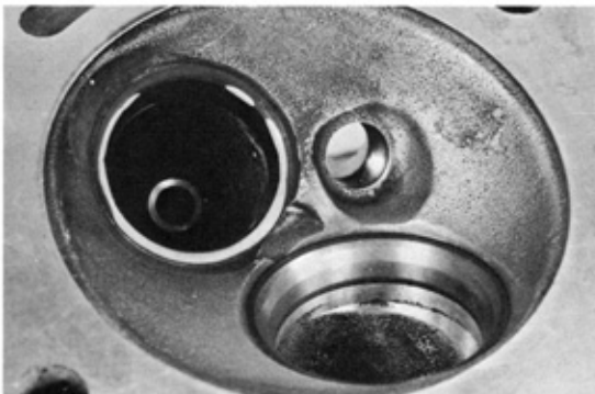
Fig. 3-60 Check Seat/Guide Concentricity
