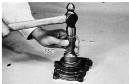
Fig. 3-179 Replace Front Seal
