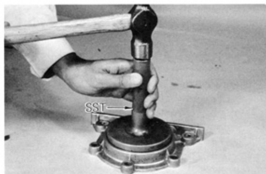
Fig. 3-180 Replace Rear Seal
