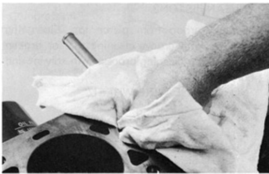
Fig. 3-144 Degraze and Clean Cylinders
