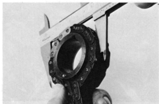
Fig. 3-115 Measure Chain and Sprocket Wear
