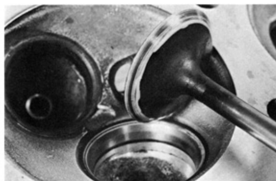
Fig. 3-57 Locate Valve Contact
