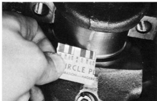
Fig. 3-156 Measure Main Bearings
