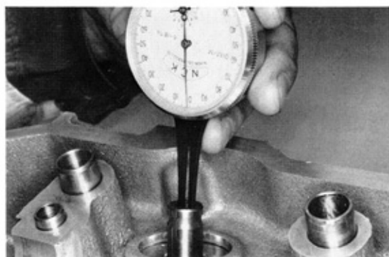
Fig. 3-47 Measure Valve Guide
