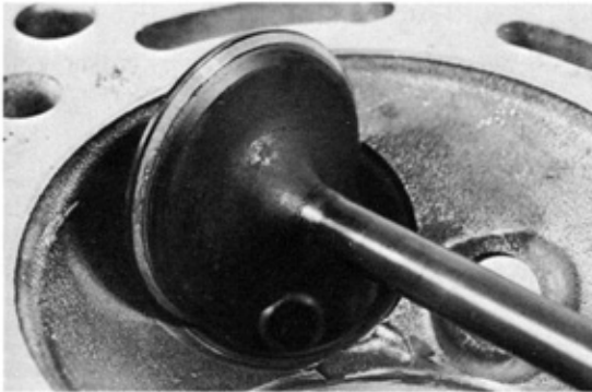
Fig. 3-59 Check Valve Concentricity
