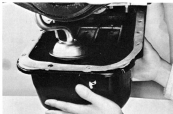
Fig. 3-103 Remove Oil Pan
