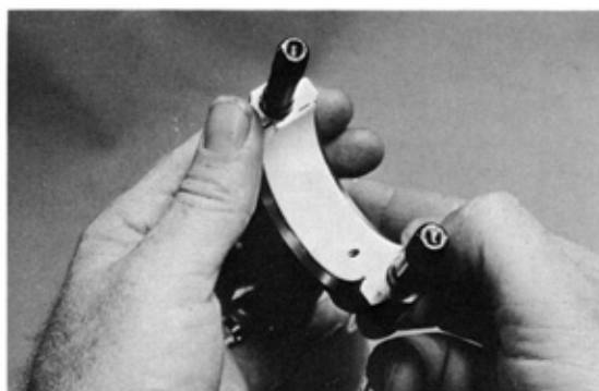
Fig. 3-161 Install Bearing Inserts
