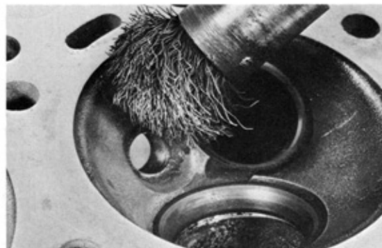
Fig. 3-38 Clean Combustion Chamber
