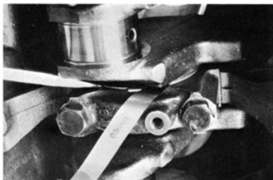
Fig. 3-154 Measure Crankshaft Thrust
