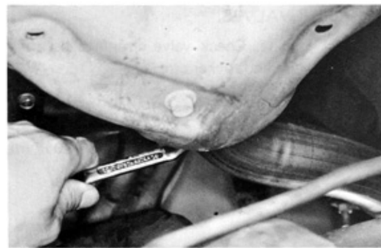
Fig. 3-97 Install Exhaust Pipe
