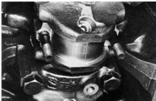
Fig. 3-137 Measure Rod Pin Oil Clearance
