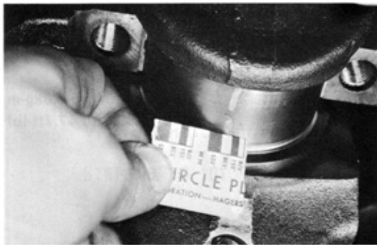
Fig. 3-159 Check Oil Clearance
