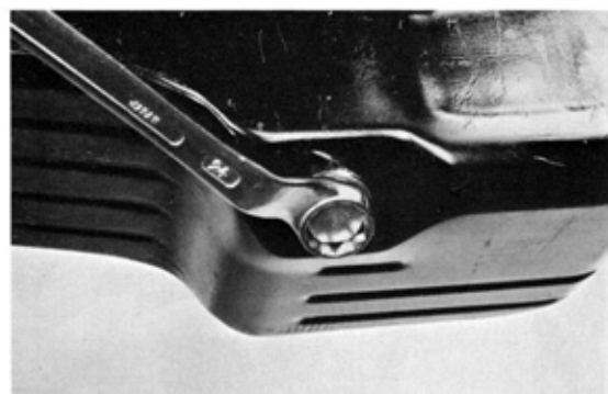
Fig. 3-21 Drain Engine Oil
