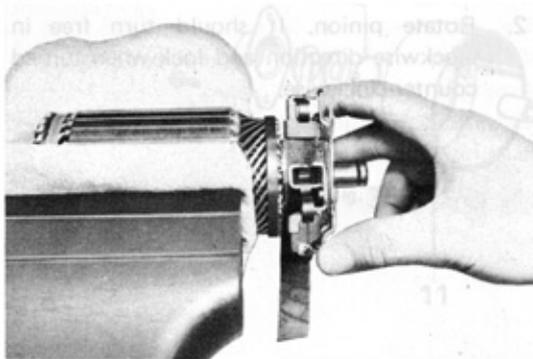
2. If brush is replaced, dress it with emery cloth to provide proper contact.
