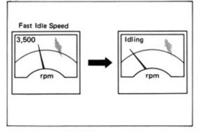
Adjust the fast idle speed by turning the fast idle adjusting screw.
