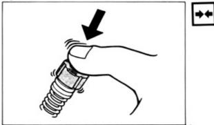
Set to the idle speed by screwing in the (5) idle mixture adjusting screw. Idle speed: 650 rpm
