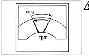
Race the engine momentarily with the accelerator link to verify that the engine returns to specified rpm when released.
