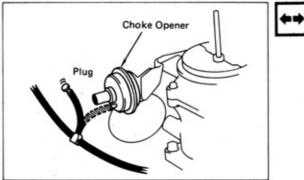
Disconnect the vacuum hose from the choke opener and plug the hose end.
