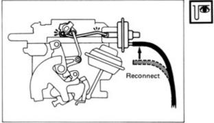
Choke valve should be fully open when the choke knob is fully returned.
