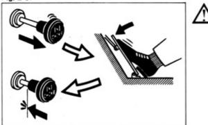
Fully pull out the choke knob, depress the accelerator pedal once, and return the choke knob about half way.
