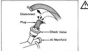
Australia N.S.W & Victoria only: З. Disconnect the air injection hose from the Al check valve and plug the check valve.
