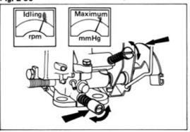
Break the idle limiter cap on the idle mixture adjusting screw if installed.
