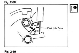
Check that the fast idle cam is at the second stop.
