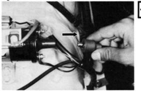
Disconnect the high tension cord from the ignition coil to cut off the secondary circuit.
