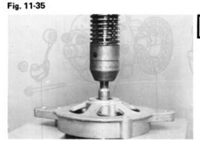
Remove the rotor from the drive end frame with a press.
