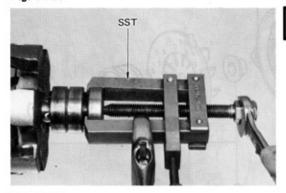
Remove the rotor shaft rear bearing with SST. SST[09286-46011]
