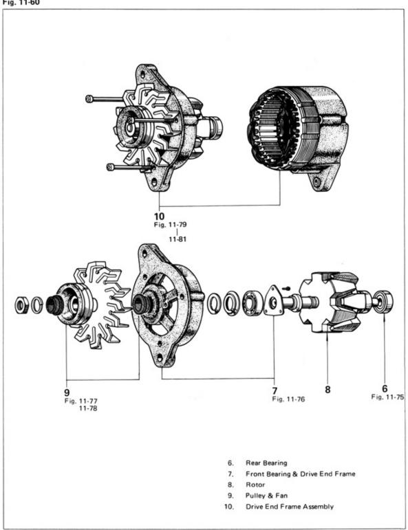
Assemble the parts in the numerical order shown in the figure.
