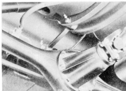
Fig. 5-3 Removing Upper Control Arm
